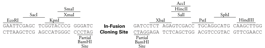
pUC19 Linearized Vector Map and Multiple Cloning Sites (MCS).
