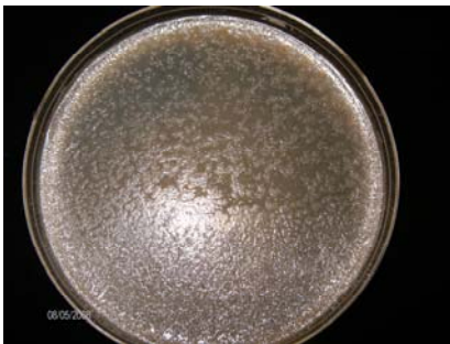
Classified as a ONE – Crystals clearly visible on surface of agar; little degradation occurring because no clear zones
